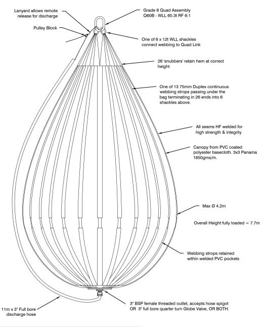
UNIQUE SEAFLEX 50t WATERLOAD BAGS ARE SUPPLIED COMPLETE AND READY FOR USE IN TRANSIT CASE FROM WHICH THEY CAN BE HOISTED WITHOUT ANY SITE HANDLING.
